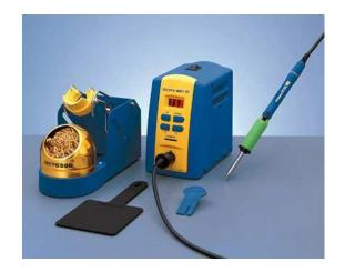
sleep mode of 0-29 minutes or auto-power shut off at 30 minutes. The sleep mode reduces the tip temperature to approximately 200°C (400°F) after the programmed time (0-29 minutes). The lower tip temperature will reduce oxidation of the tip and improve the tip performance. When in sleep mode the tip will quickly return to temperature after the iron is removed from the holder.
